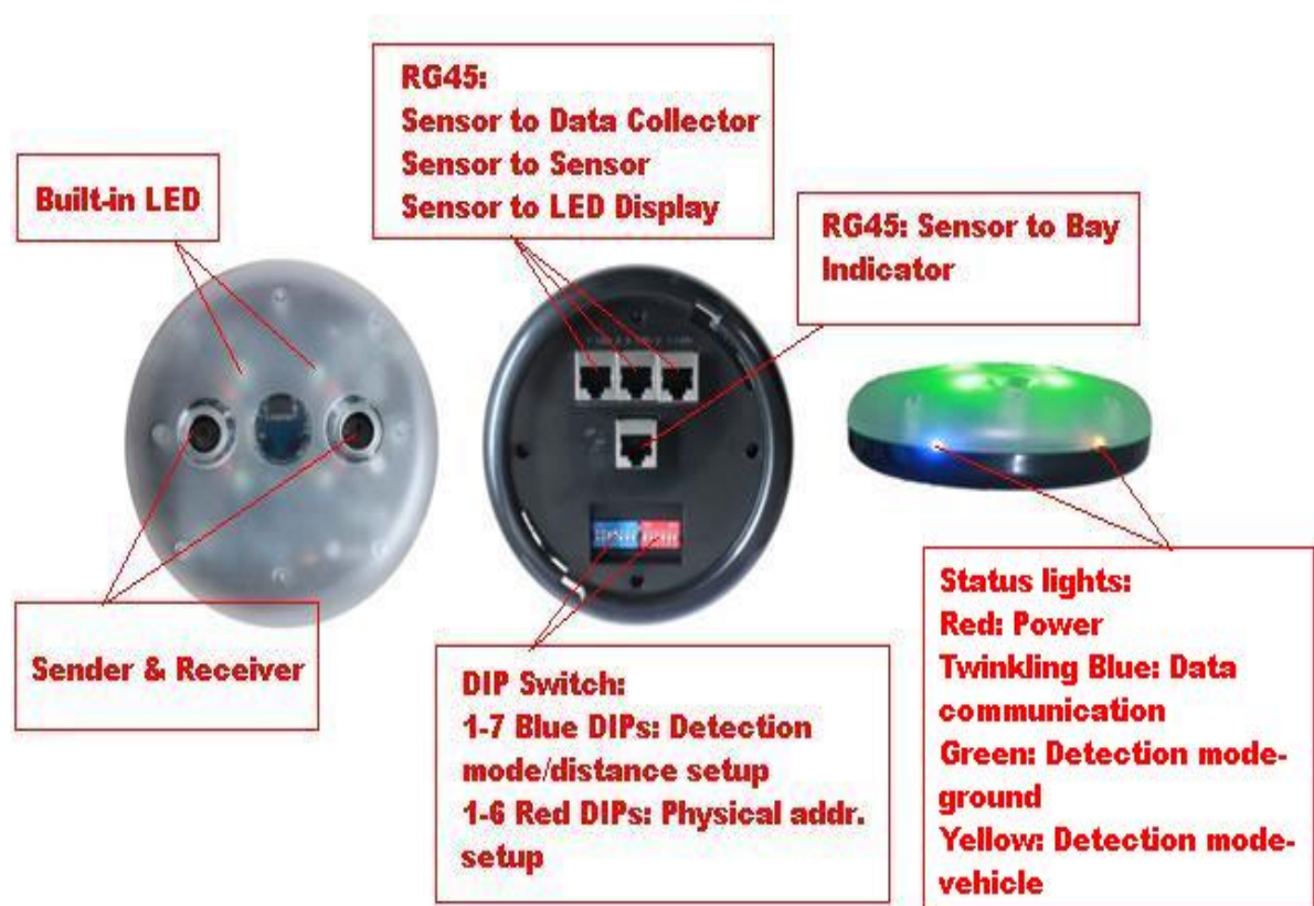
Picture 3 – Ultrasonic Sensor
